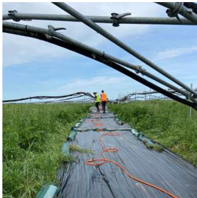
Figure 3: An ERT (Electrical resistivity tomography) experiment to quantify landfill water content.
